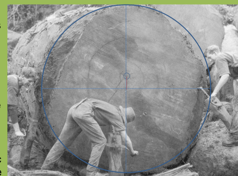
Figure 6: Historical Photograph of a kauri cross-section. The blue line and circles shows the circumference, geometric centre, and the location of the pith. These were used to calculate the eccentricity ratio for this cross-section. The red line is used to calculate the distance from the geometric centre to the pith. Source: The Kauri Cameraman.
