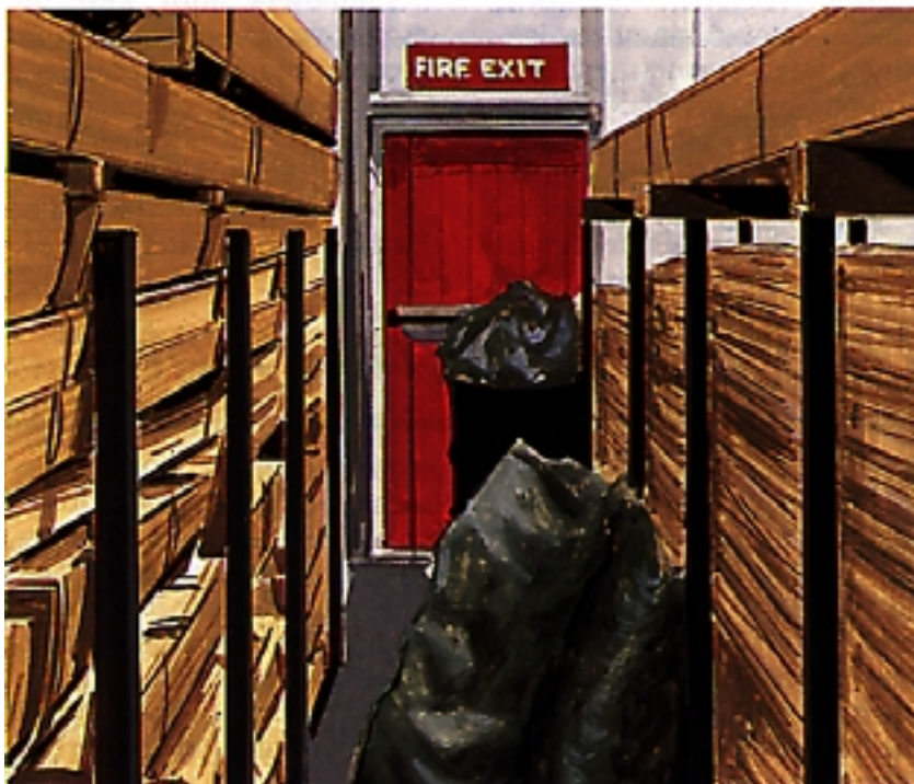
Fire exits must never be blocked
