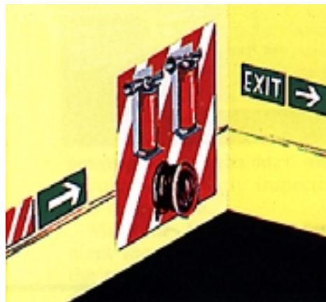
Fire-fighting equipment and emergency route sign
