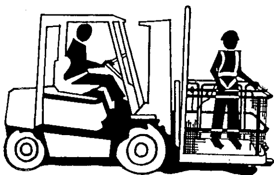
Fig. 23 An example of an engineer-designed man cage, with safety harness and lanyard assembly, correctly positioned on forklift tynes
