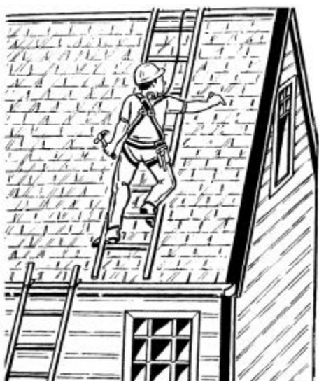
Fig. 19 Bracket on roof ladder should reach over the ridge
