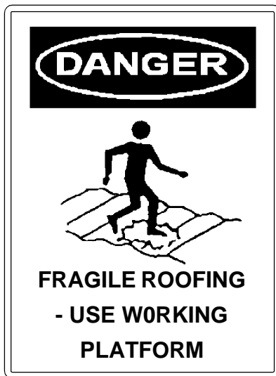
Fig. 36 Danger signs to be fixed at points of access to the roof
