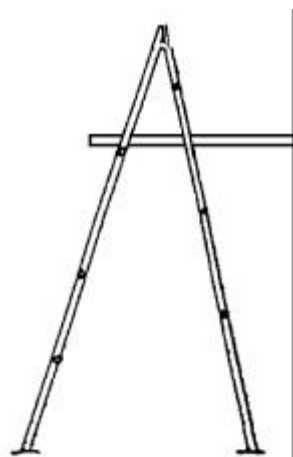
Fig. 18 Light-duty trestle. Maximum height: 3 m; maximum loading: 160 kg
