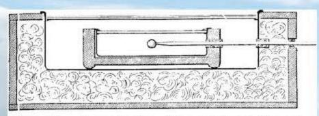
Cross-section of Langley's hot box, which was similar to de Saussure's later models. A thermomether penetrating the walls at right was used to measure the air temperature inside the inner box.
