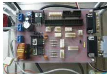
Figure 8. The new power distribution board
