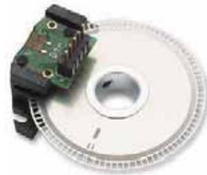
**Figure 2.** An optical encoder
