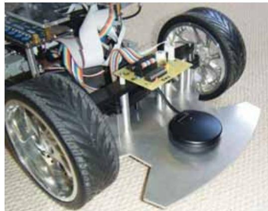
Figure 5. The position of the GPS on the AVG
