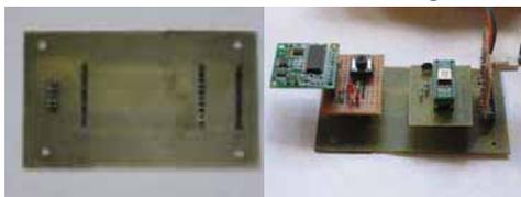
**Figure 2.** Routing Board PCB
