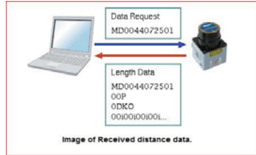
Figure 3: A data request from host pc to the Laser Range Finder (LRF) (Reproduced from [6])
