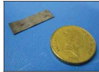
Figure 1. IPMC strip used in this project. A NZ$1 coin is used for size comparisons.
