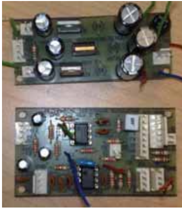
Figure 1. Printed circuit boards containing the power supply circuit (top) and the amplification circuit (bottom)
