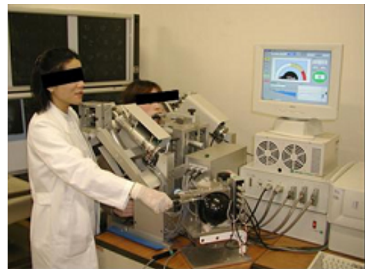
Figure 7. The jaw training with WY-6 robot [10]
