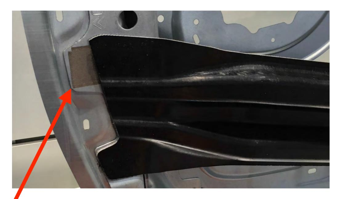
• Joining - Microstructuring of surfaces allows better gluing of different materials.
