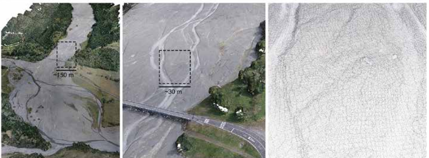
Figure 1 - An example of point cloud data on the Tapuaeroa River. The point density achieved was close to 25 pts/m 2 , along a 12.5 km transect of valley floor. Fine details of river morphology are resolved, such as abandoned channels and bar-top sheets of fine sediments. Even grain roughness can be resolved, in coarser sediments.
