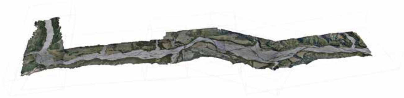
Figure 2 - Merged point cloud, representing five surveys, with over 160 million data points, generated using 2,700 photos.
