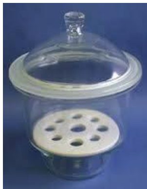
Desiccator Used for store material and protect it from air contamination or humidity
