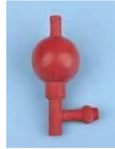
Pipette bulb Used along with pipette to suck liquid
