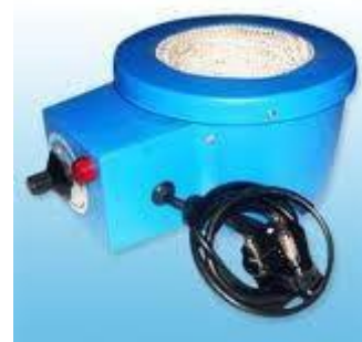
Heat Mantle Used as source of heat, mainly for distillation system
