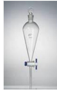
Separation funnel Used for liquid-liquid extracts, for increase separation efficiency
