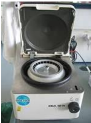
Centrifuge Used for separation of precipitations from supernatant
