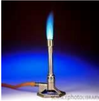
Bunsen burner Used as heat source
