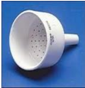
Buchner funnel Used for vacuum filtration using filter paper
