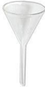
Glass funnel Used for liquid transfer. Also for simple filtration
