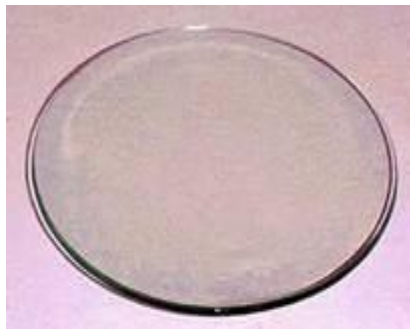
Watch glass Used for evaporating liquids, covering beakers, or as a weigh boat
