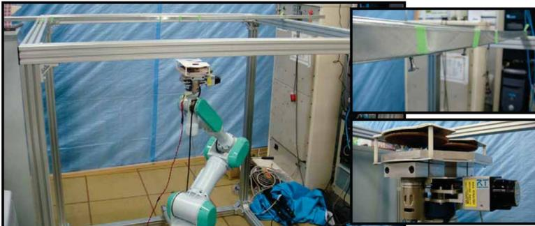
Test setup for the screw removal robot system.
