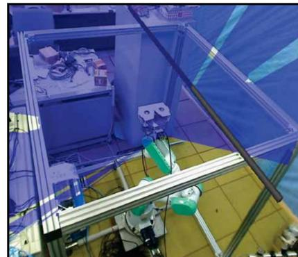
An Augmented Reality (AR) view of the robot in action. The virtual ceiling beam is shown placed over the robot.
