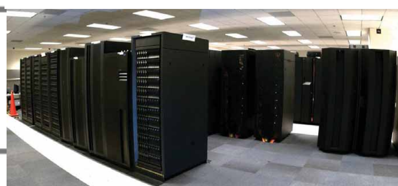
The BeSTGRID computer cluster at The University of Auckland is a parallel machine with > 100 processors and > 500 GB of memory. This setup makes it ideal to run our parallel FDTD code; without BeSTGRID this research would not be possible:
