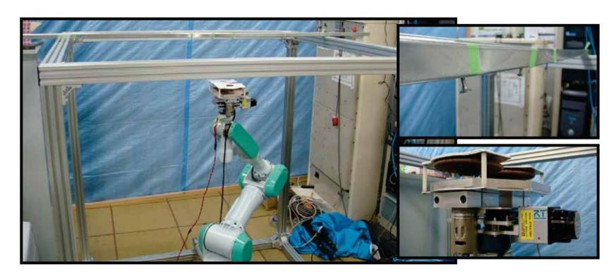
Test setup for the screw removal robot system. Right: Ceiling beam with screws, and the custom screw removal tool.
