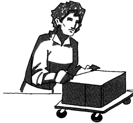
Fig 18 Rolling platform to avoid lifting
