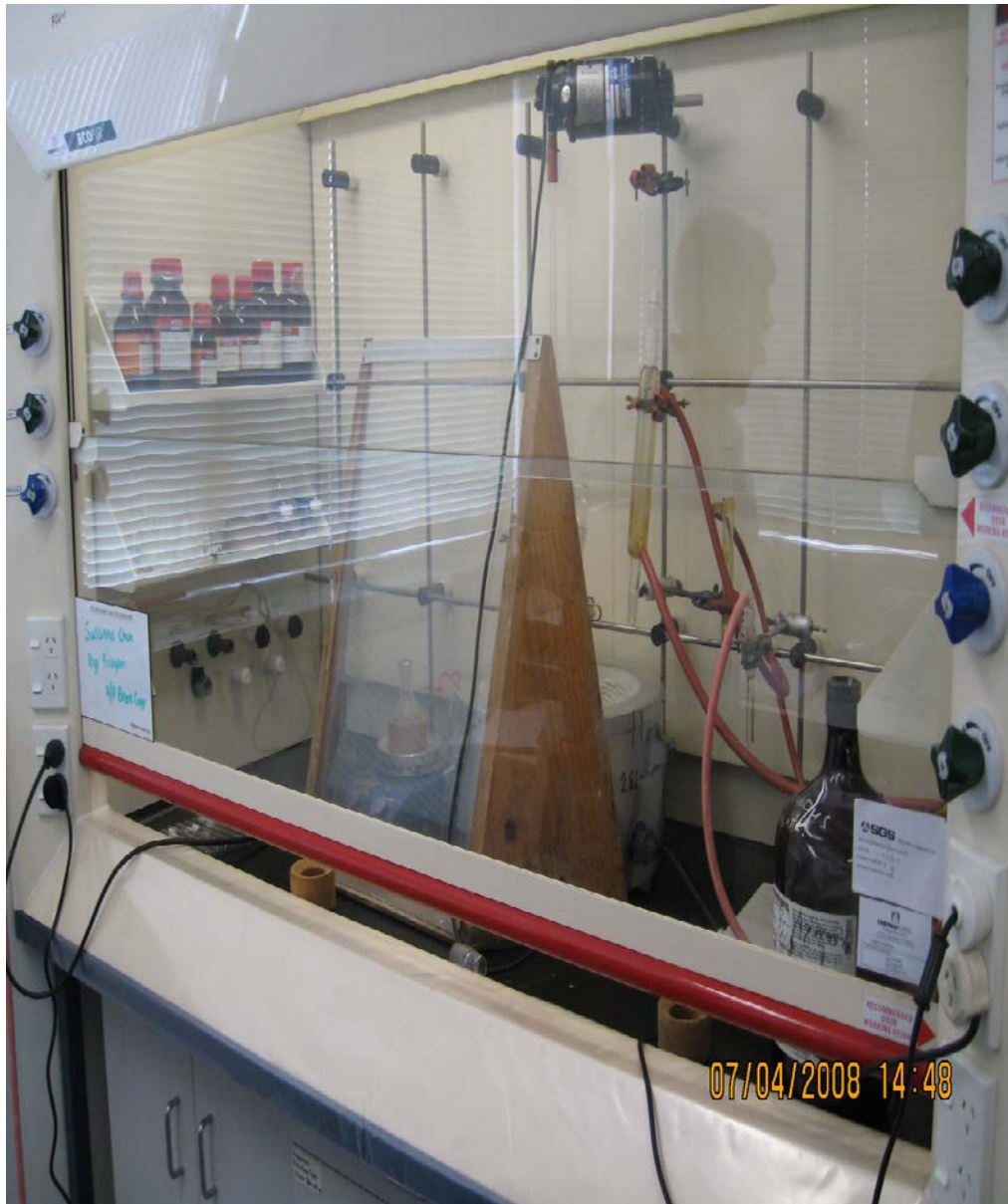
Ideal use and set up of a Blast Shield. Note that the combination of fully lowered fume hood sash and Blast Shield assist in containing any potential explosion.
