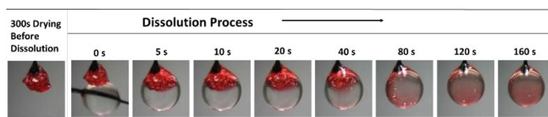
**Figure 2.** Dissolution Process for GA encapsulated cranberry juice particle
