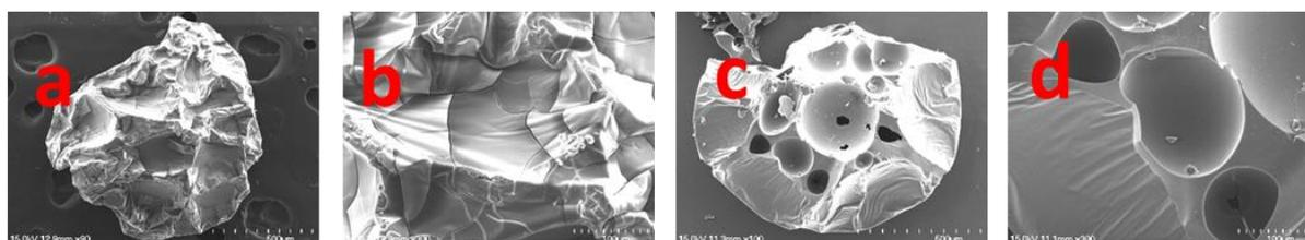
**Figure 3.** SEM images of dried cranberry particle encapsulated with GA. (a) Surface (90 $\times$ ) (b) Surface (300 $\times$ ) (c) Cross section (100 $\times$ ) (d) Cross section (300 $\times$ )
