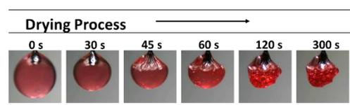
**Figure 1.** Drying Process for cranberry juice encapsulated with GA
