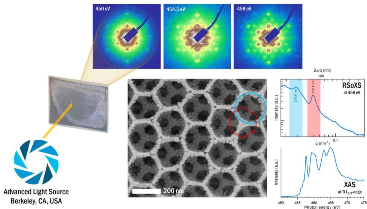
**Figure 1.** (Top) RSoXS images collected at various X-ray photon energies over the Ti L<sub>2,3</sub>-edge. (Centre) SEM image of a TiO<sub>2</sub> inverse opal, showing a *fcc* array of macropores. Coloured shapes corresponding to scattering features seen in the reduced RSoXS pattern collected at 458 eV (right).
