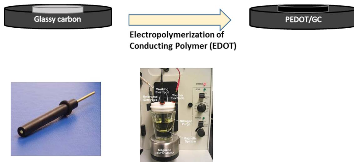
**Figure 1.** Electrodeposition of PEDOT on the glassy carbon electrode surface using cyclic voltammetry.
