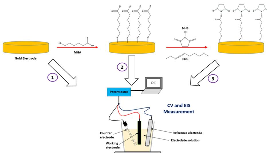
**Figure 1.** Stepwise surface modifications of a gold electrode suitable for chemical and biological sensing and electrochemical measurements at each step.
