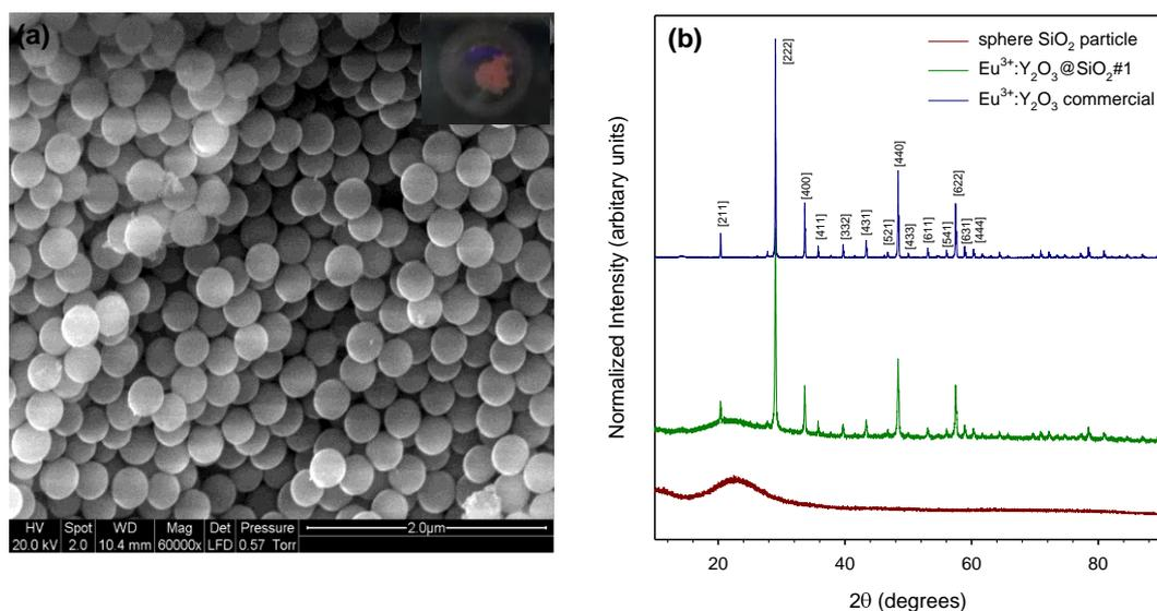
**Figure 1.** (a) SEM image of the  $\text{Eu}:\text{Y}_2\text{O}_3@\text{SiO}_2$ . The inset shows the luminescence of  $\text{Eu}:\text{Y}_2\text{O}_3@\text{SiO}_2$  under 365 nm excitation (b) XRD data for the  $\text{SiO}_2$  core,  $\text{Eu}:\text{Y}_2\text{O}_3@\text{SiO}_2$  and a commercially available  $\text{Eu}:\text{Y}_2\text{O}_3$  powder.
