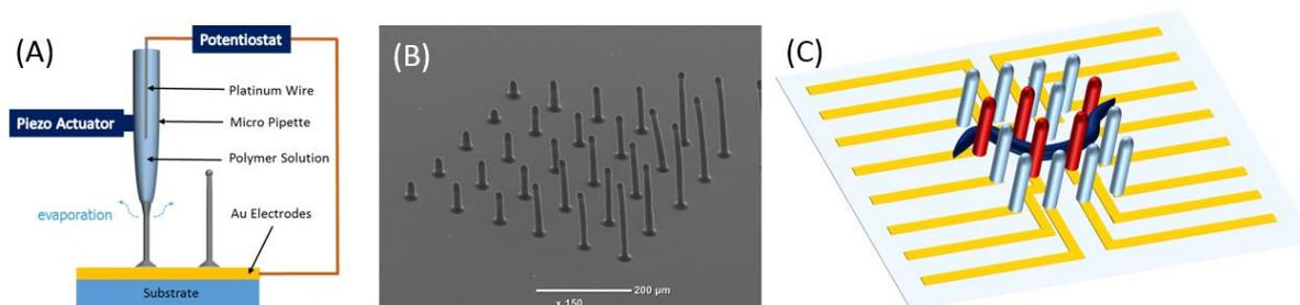
**Figure 1.** (A) Schematic mechanism of direct writing. (B) SEM of CP array. (C) Applications of CP arrays for *C.elegans* sensing and stimulation<sup>2</sup>.
