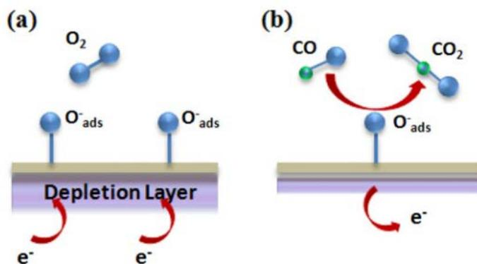
**Figure 1.** Illustration of  $n$ -type semiconductors: (a) adsorbed oxygen (b) reducing gases released.<sup>3</sup>
