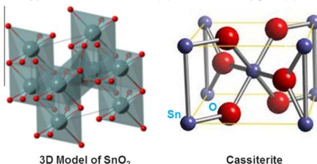
**Figure 2.** 3D model of tin oxides ( $\text{SnO}_2$ ).<sup>4</sup>
