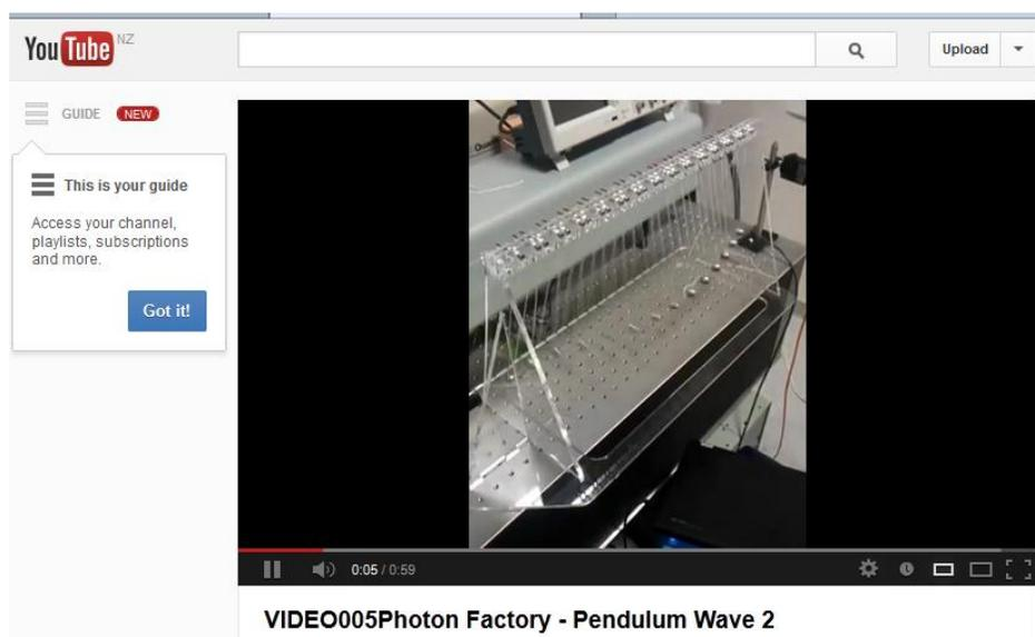
*Pendulum wave demonstration built in response to student suggestion. Students time the wave oscillations.<sup>5</sup>*
