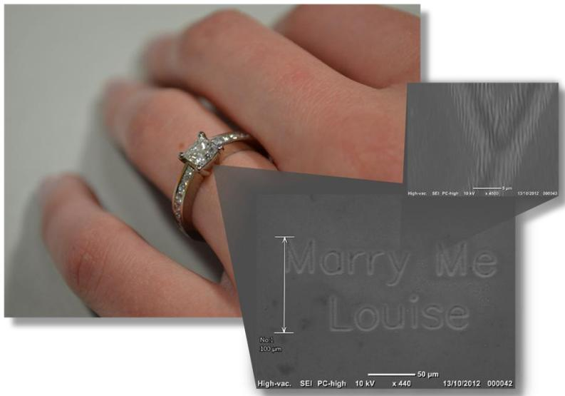
*Jake proposed using the laser to write letters smaller than a grain of sand on the ring. She said “yes!” We used the same technology to write “Poetry off the Page.” (below)*
