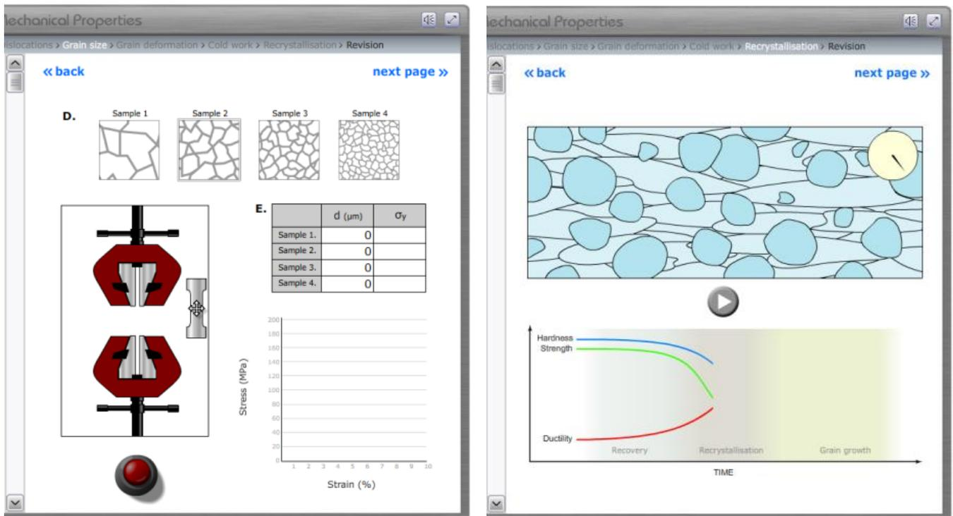
**Screen grabs from “Microstructure and Mechanical Properties” showing a virtual tensile test (L) and an animated “recrystallization”.**
