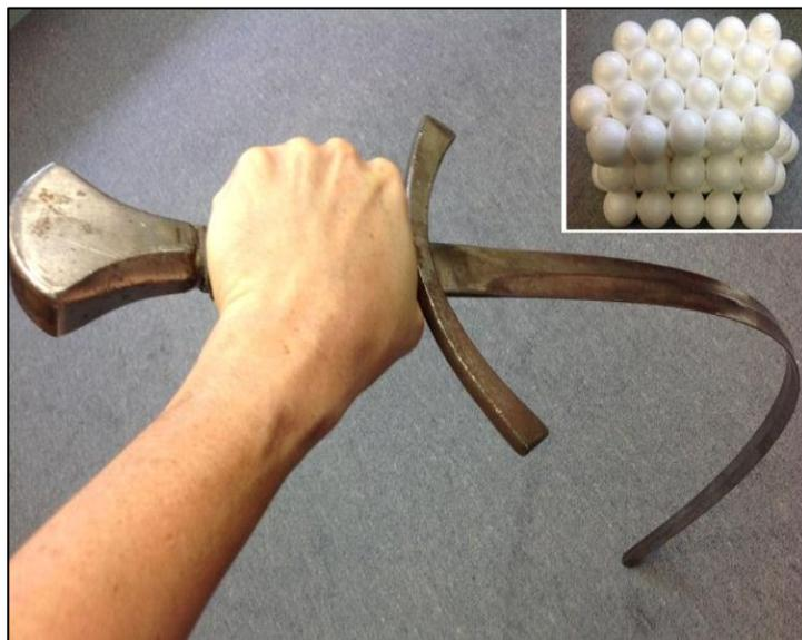
*“May your swash never buckle”. The elastic deformation of a sword and a model of atoms used to explain it.*
