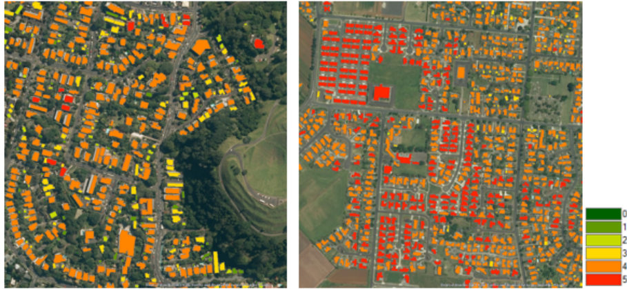
Figure 4: Results from rating rooftops based on the annual solar radiation on the 14 \text{ m}^2 with the highest results in an older suburb (left) and a more recently built suburb (right).
