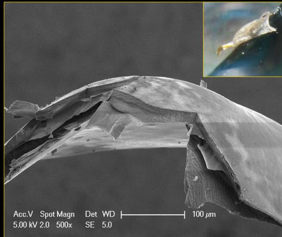
All layers in the chirped structure have thicknesses on the same order as visible light wavelengths (100-700 nm), which results in broadband reflection over the visible to near-IR regions. This is schematically shown to the right.
