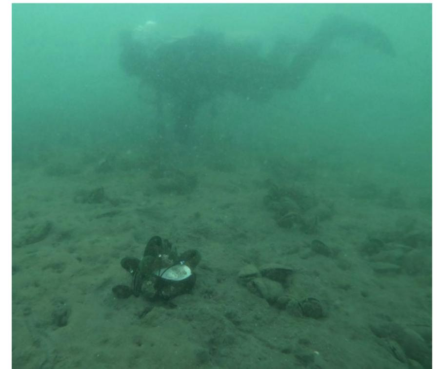
Gape sensors deployed on mussels on a restored mussel bed.
