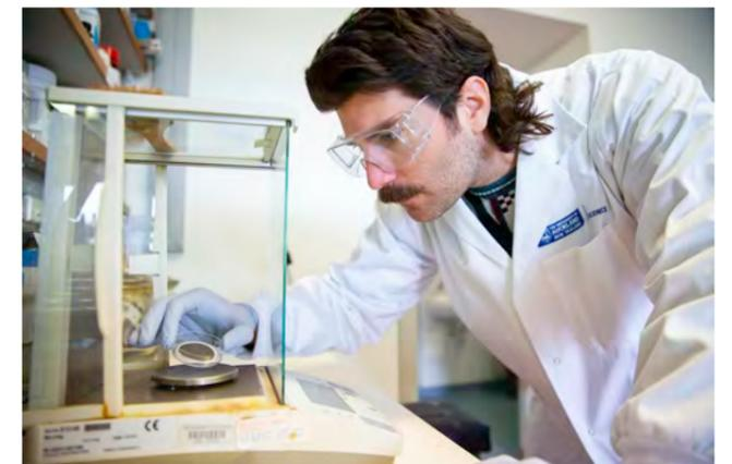
Dr Joel Rindelaub weighs out filters on the analytical balance to perform gravimetric analysis of aerosol mass loading. Photo: Elise Manahan
