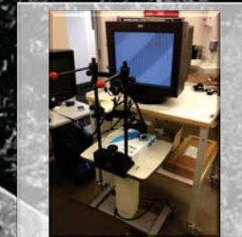
Figure 4. The Arlington ViewPoint eye tracker 400Hz Binocular Real-time Torston used in the study
